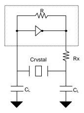
$C_L = 2^*(C_P - C_S),$  Where  $C_P = \text{Load}$  capacitance of crystal
